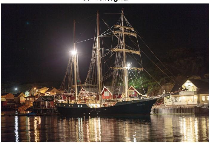
The SV *Antigua* was built in 1957 in Thorne (UK) and served for many years as a fishing vessel, until it was completely re-built in the early 1990s in the Netherlands as a barkentine and equipped as a passenger ship. A barkentine has three masts with square sails on the foremast.
